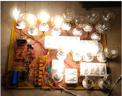
Fig. 5 Shows load is increased so that in order to limit the maximum demand low priority load tripped (Bulbs in last row).
